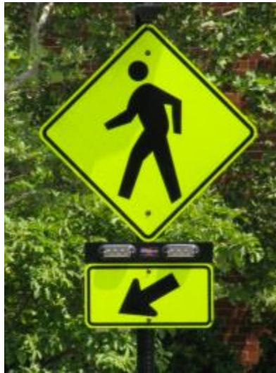
Figure 23. Rectangular Rapid Flashing Beacon. (Source: Carol Kachadoorian).
