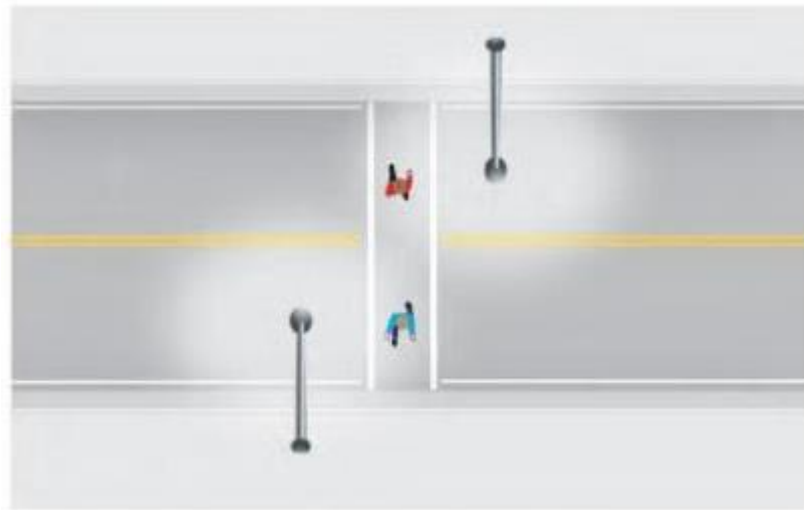
Figure 18. Proper placement of pedestrian-scale lamp posts provides illumination for the crosswalk. (Source: Michele Weisbart for the Model Design Manual for Living Streets).
